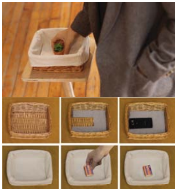
Figure 5. A demonstration of how the smartphone is triggered with an object, and how it is embedded inside the basket with a cloth.
